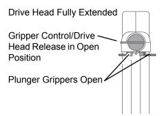
Insert syringe (from front of instrument) by sliding flat edge of syringe barrel flange between barrel flange grippers.
