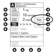
7. To enter loading dose, press **LOAD DOSE** soft key, press **Yes** soft key and use numeric data entry keys.
