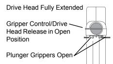
7. Insert syringe (from front of instrument) by sliding flat edge of syringe barrel flange between barrel flange grippers.
