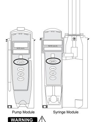
Ensure that the displayed syringe manufacturer and syringe size correctly identify the installed syringe. Mismatches might cause an under-infusion or over-infusion to the patient that could result in serious injury and/or death. For a list of compatible syringes, see "General Information," "Compatible Syringes."
