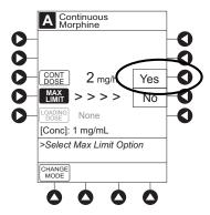
To enter loading dose, press **LOAD DOSE** soft key, press Yes soft key, and use numeric data entry keys.
